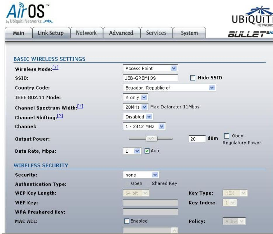
The screenshot displays the AirOS configuration interface for a Ubiquiti Bullet 2HP device. The interface is divided into two main sections: "BASIC WIRELESS SETTINGS" and "WIRELESS SECURITY".
